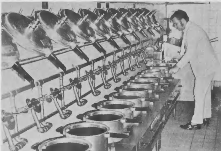
The modern kitchen is equipped with, among others, fourteen large pressure cookers.
